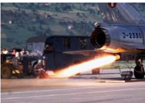
Mirage IIIS: Ground test with liquid propelled rocket booster SEPR; Photo: Peter Gunti
