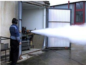
SHWR1.2k-I produces a thrust of 120kg
