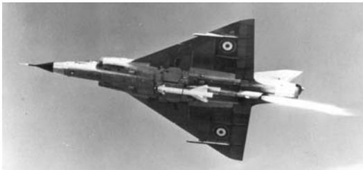
Figure 11 : SEPR 841 ignited on Mirage III C
