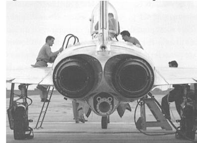
Figure 8 : Rear view of the MD 550 showing the engine arrangement
