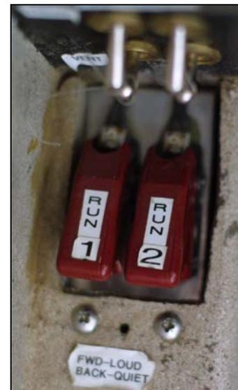
**Figure 9. Very simple engine control interface for pilot.**
