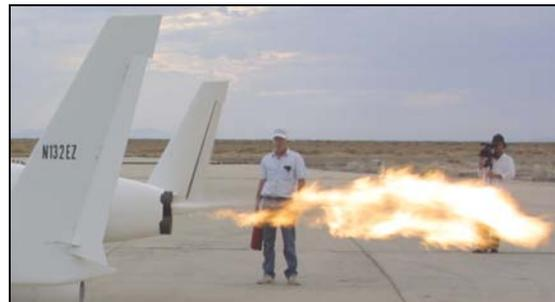
**Figure 5. Cascaded purges in action. Residual propellants are safely blown out of an engine at shutdown.**
