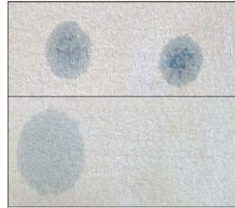
**Figure 6. Jet-A, left, vs high grade kerosene on right. High grade kerosene evaporates completely in 10-20 minutes.**
