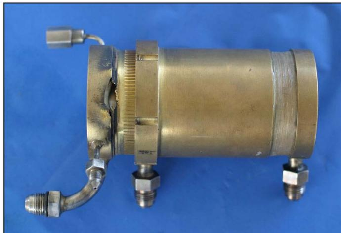
**Figure 7. Why flame-to-world seals are to be avoided. Chamber and injector damaged by escaping flame. (Jacket pulled back to show detail.)**
