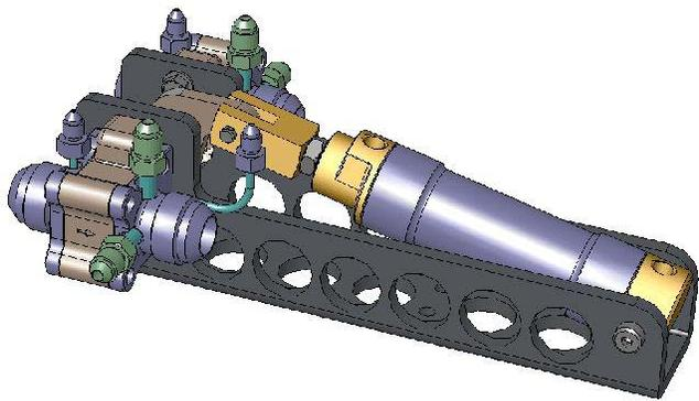
**Figure 4. Ganged-actuator LOX-fuel valves with purge and igniter tapoff ports, using COTS cryo-rated valve components.**
