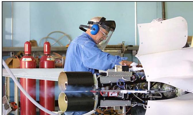
**Figure 11. Mechanic wearing face shield, hearing protection and gloves loads liquid oxygen into EZ-Rocket.**
